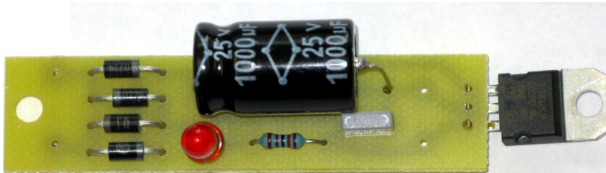
12 Volts AC to 12 Volts DC rectifier inside the viewer.
